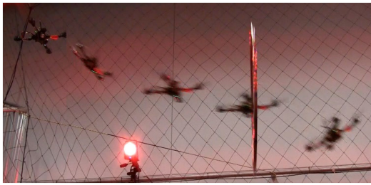
Fig. 5. Composite image of a single quadrotor flying through a thrown circular hoop. See attached video or http://tinyurl.com/pennquad .
