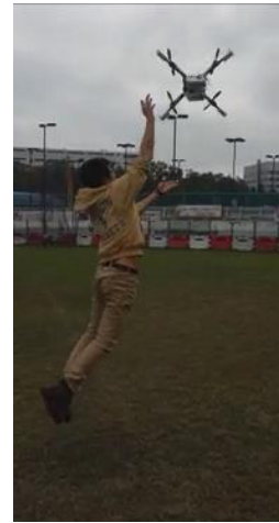
Fig. 9: Our UAV can be thrown up and start to hover autonomously
